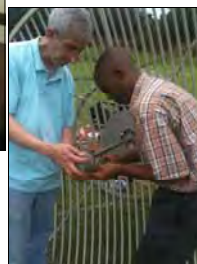
Training their technician in the use of test equipment and how to check a microwave dish.
